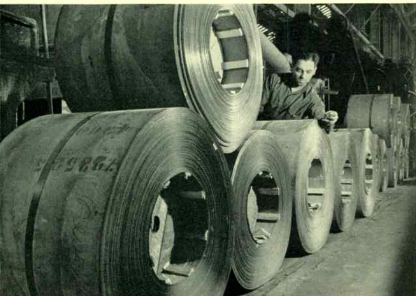
Rolls of Hipersil ready for slitting into ribbons, which are wound into transformer cores. Hipersil is a new material that has one third more flux carrying capacity than the best grade of hot-rolled silicon steel.
