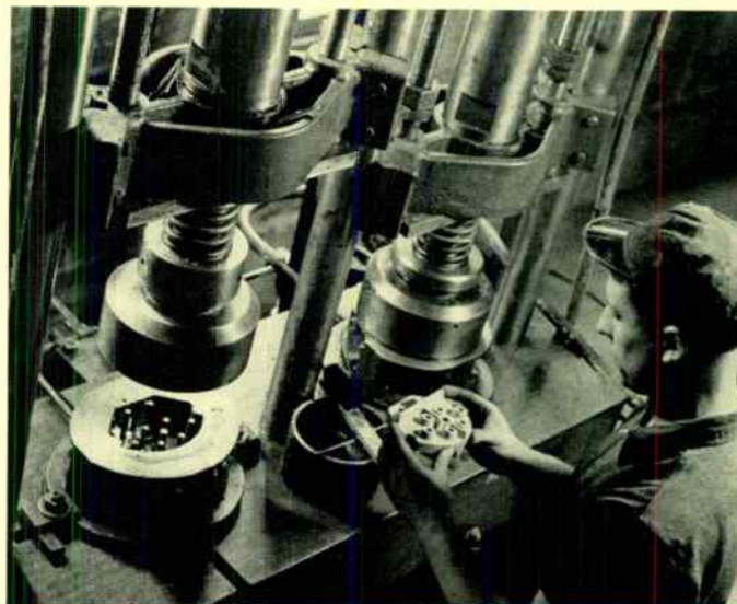
Prestite, a porcelain made by a new method, possesses the superb electrical qualities of wet-process porcelain and the dimensional fidelity of that made by dry process.
