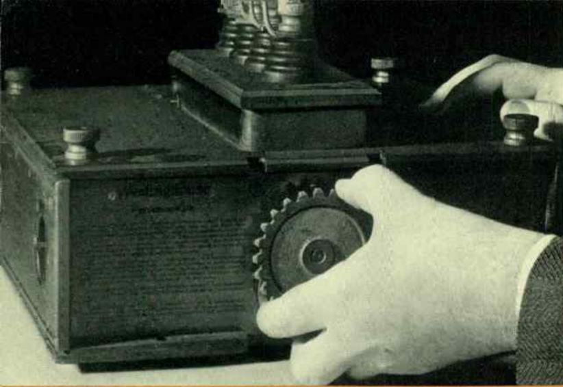
Fig. 6—Klydonographs such as this were used to record arc-furnace surges. The device was developed about twenty years ago and played a leading part in the early field studies of lightning. It consists of a grounded metal drum, covered with a Micarta cylinder about 0.1 inch thick. A clockwork mechanism drives the drum and draws a photographic film over it in a fashion similar to a roll-film camera. Insulated metal electrodes bear on the surface of the film and are connected to the points where surge voltage measurements are desired. The surge magnitude is found by measuring the diameter of the familiar Lichtenberg figure.
