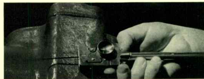
Vibrating-reed frequency indicator.
