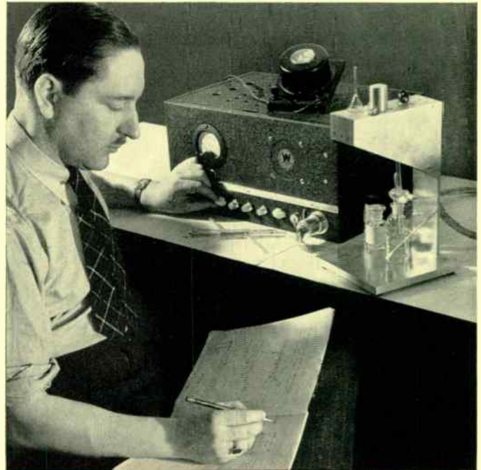
Demand for Geiger counters, created by increasing usefulness of artificially radioactive substances, has resulted in factory-made units no larger than a table radio.
