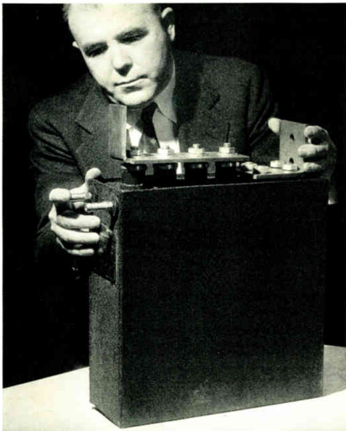
This capacitor, the size of a 15-kva 60-cycle unit, can handle continuously 230-kva (766 amperes, 300 volts) at 11 520 cycles.
