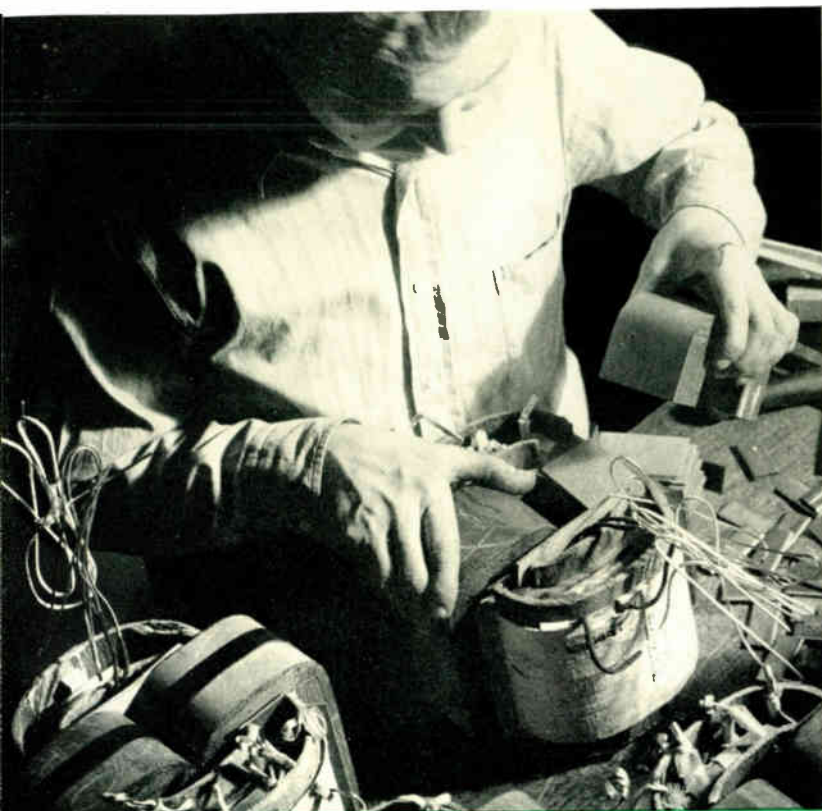
Fig. 9—For small distribution transformers the core is made of wound Hipersil instead of stacked laminations. After impregnating with a bonding material the core is cut in two so the machine-wound core can be slipped over the iron. The core halves are again joined and held in position by straps, as can be seen on the core and coil assembly in the lower left corner.
