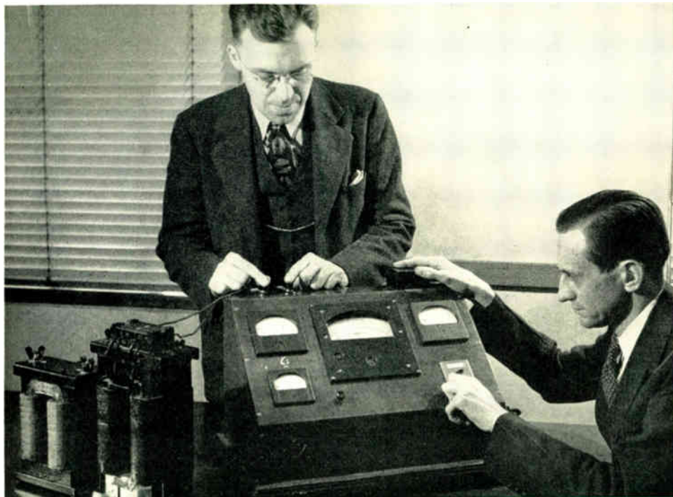
Fig. 5—Demonstrations of the bearing of the greater permeability on core size and weight. The test cores at the left have the same iron loss, exciting current, and copper resistance, but the one at the left is made of Hipersil, the one at the right of high-grade ordinary silicon iron. The silicon L-plate core weighs 38\frac{1}{4} pounds; the Hipersil core weighs 21\frac{1}{4} pounds.
