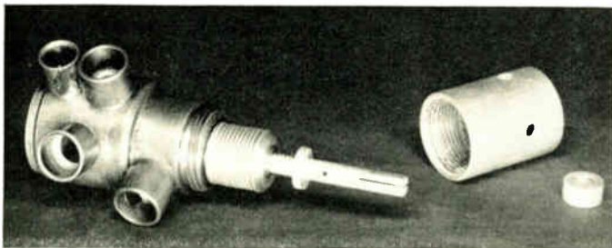
Fig. 7—The valve that reverses the cycle in the window-type unit.
