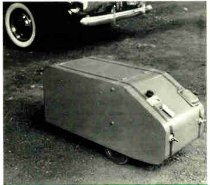
What looks like a typewriter case, or a toy tank, is a real portable welder. Small in size, it is nevertheless capable of performing work comparable with its big brothers.
