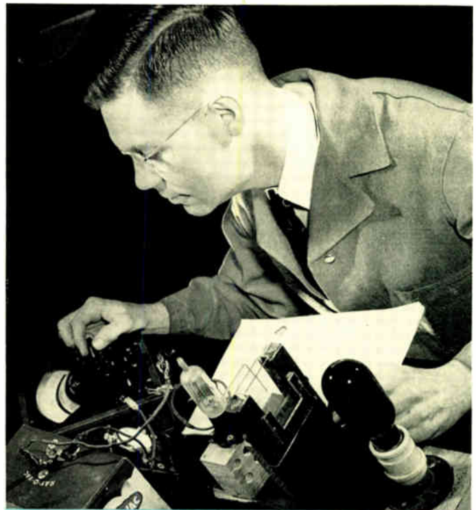
From the microammeter reading, Dr. Beese can determine the reaction of the fluorescent canary glass to the ultraviolet rays emitted by the black lamp at the right. A quartz water cell removes the unwanted infrared rays before the light impinges on the photocell.
