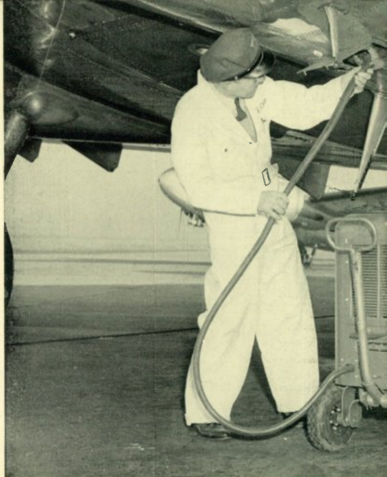
Copper-oxide rectifiers have taken over the job of starting airplane engines.
