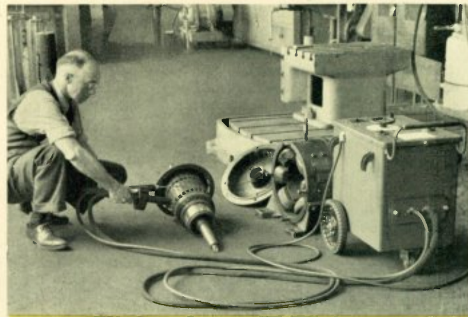
The new portable high-voltage insulation tester provides a convenient means of on-the-site testing that saves time and labor. It can be controlled at the set and at the end of the long leads.
