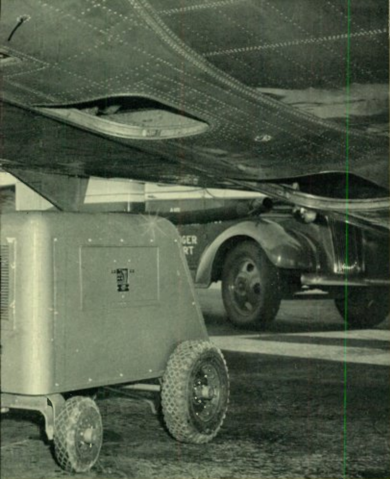
Thus power is used from the airport system instead of from batteries.
