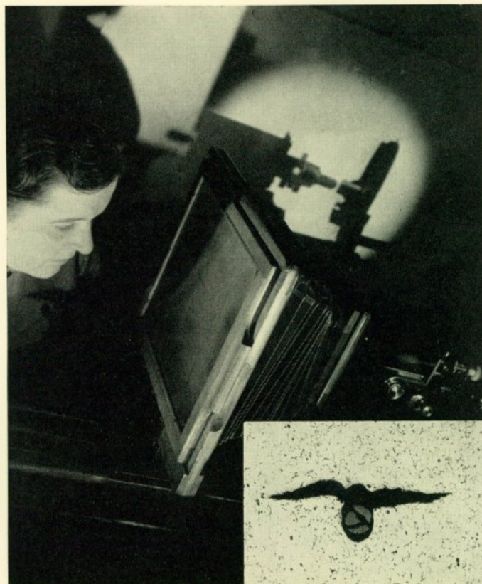
Miss Ferguson examines the polished surface of a sample by means of a microscope. The insert is a photomicrograph of an unusual flaw. Here is detailed a fractured inclusion in a fracture.
