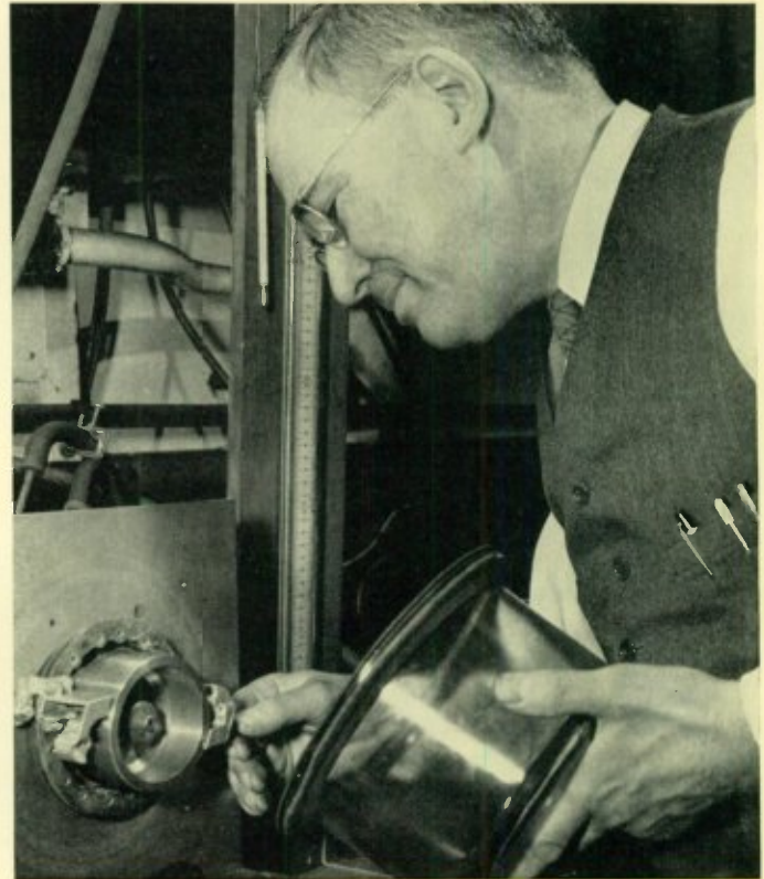
This apparatus enables Dr. Elsey to simulate the atmospheric conditions of pressure and humidity that prevail at altitudes upwards of 30 000 feet where brush wear in fighter planes has been excessive. The new type brushes are 50 times better than the old.
