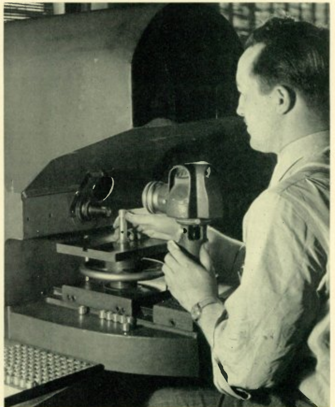
This optical comparator increases production many times with greater accuracy and without any eye strain. The size of the commutators is evidenced by comparison with the thumb of the operator. The minuteness of the segments and separators can be imagined.
