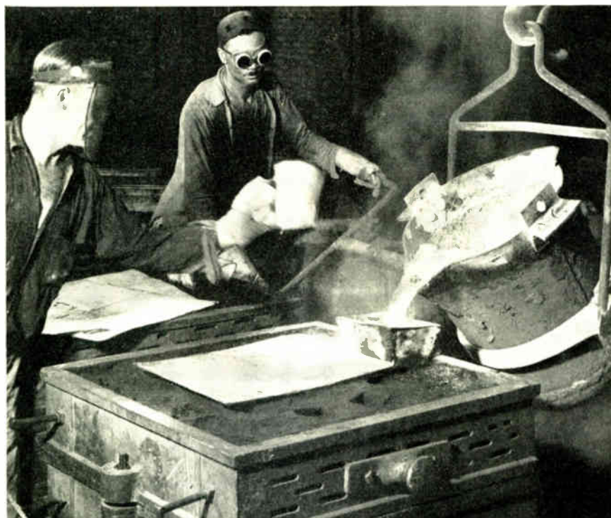
Most structural magnesium goes into castings, which do not require much change in usual foundry practices. (American Mag. photo.)
