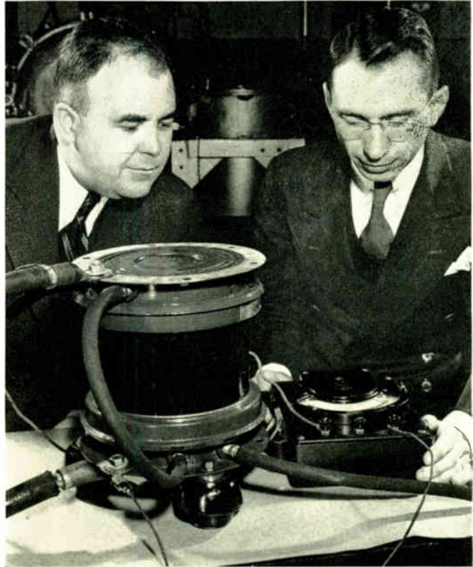
Aiding Mr. R. E. Marbury (left) in checking this new porcelain-encased capacitor in the Capacitor Laboratory is Mr. C. V. Fields. The flat plate at the end of the capacitor is for electrical contact and shows how the capacitors can be stacked or bolted to bus bars. The hose connections are made below the end plate.
