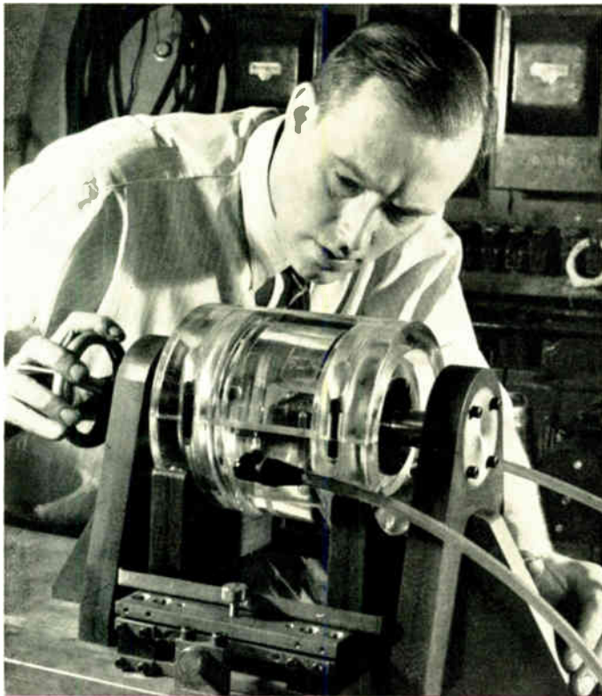
Accurately machined translucent Lucite bearings allow Mr. Boyd to see the results of lubrication design changes, and immediately. Red pigmented oil is used for clear perception.
