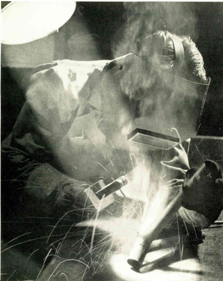
The brilliance of the light that floods the work position enables the operator to see clearly the parts to be welded and the progress of the weld itself. Heretofore, the visibility of the work position through the welder's hood has been poor, even after the arc had been struck as shown by the top inset. The middle inset shows the clarity with which the work can be seen and the arc struck at precisely the proper point. The bottom inset was taken during the welding operation and it makes a striking contrast with the top inset.
