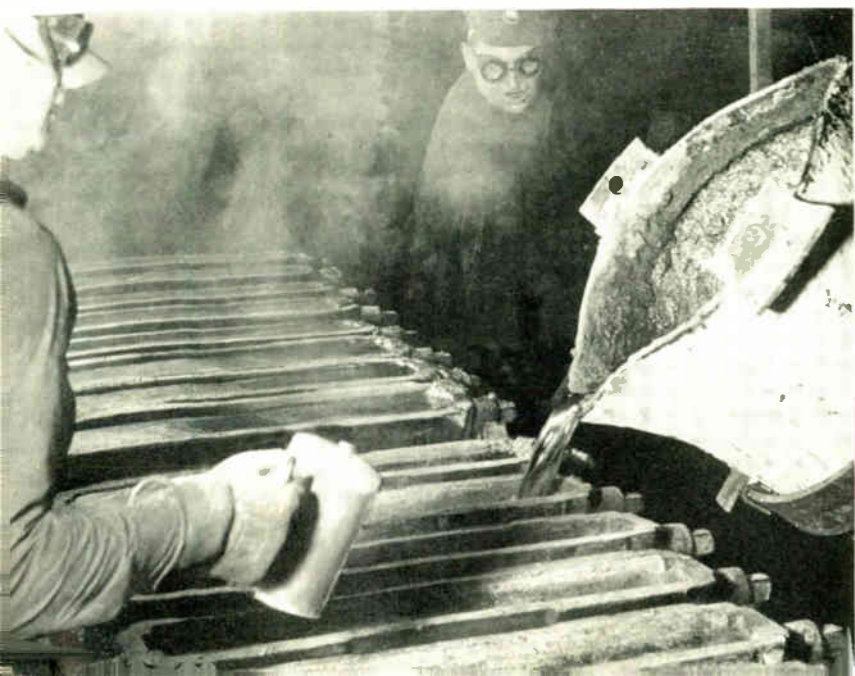
As magnesium is poured into molds for pigs a workman sprinkles the surface with sulfur dust. (American Mag. photo.)
