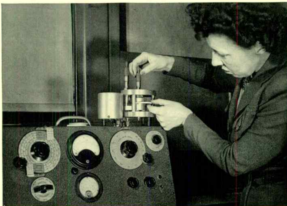
Micrometer adjustments insure accurate measurement of the dielectric characteristics of the disc-shaped sample that is placed between the plates of the holder.
