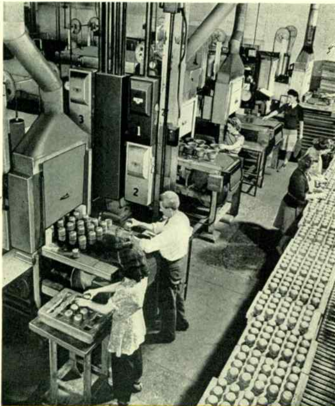
Fig. 9—A battery of four conveyor-belt controlled-atmosphere furnaces used for small brazing assemblies. Insecticide bombs are brazed in the furnace in the foreground.
