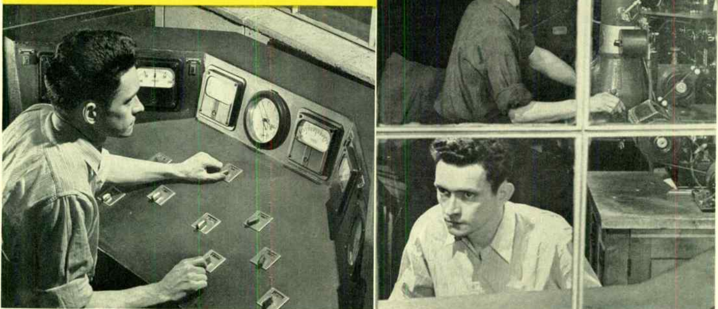
Fig. 5—All controls, indicating instruments, and recording devices are in a centralized room conveniently located to give the operators a full view of the testing area and of the impulse generator. Looking through the window from the test floor (right) one sees the operator at the control desk and behind him is the electronic oscillograph and its operator. The view below is taken looking over the right shoulder of the control-desk operator.
