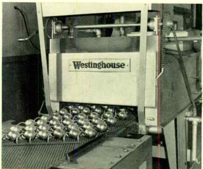
Fig. 5—A channel to support the tube ends positions the assemblies on the woven belt without elaborate supports.
