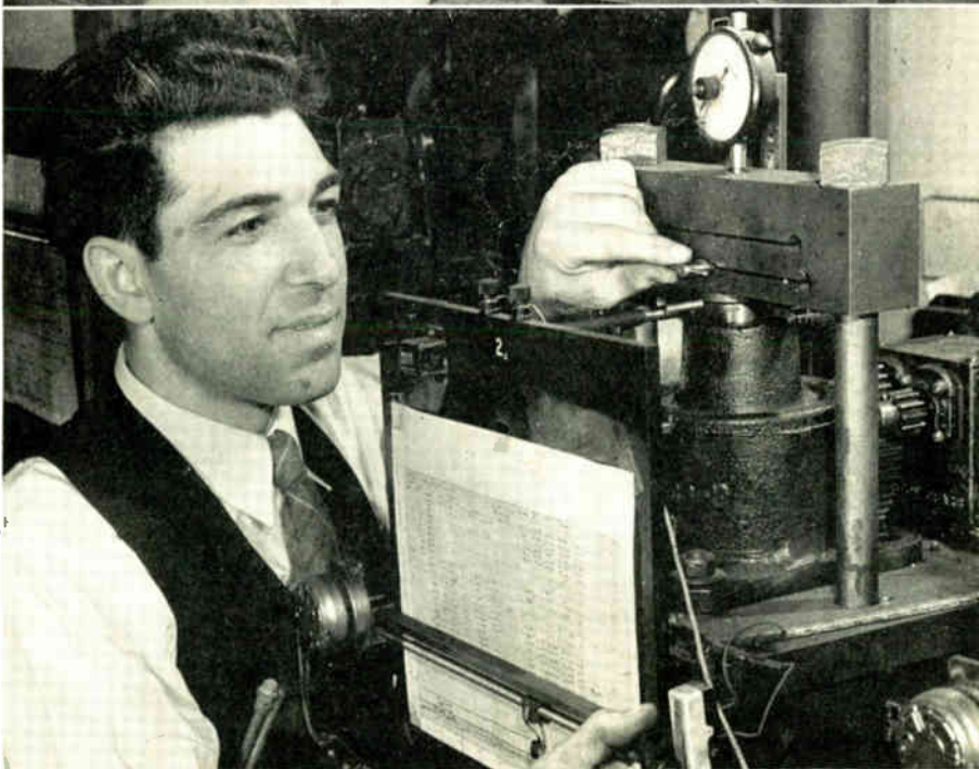
A force-measuring bar with two ranges is shown in the picture above. Pins such as shown in the foreground are placed in the holes in the slots, both in front and back of the bar. In the lower photograph, Mr. M. J. Manjoine is changing the range of a weighing bar on an automatic creep-testing machine.
