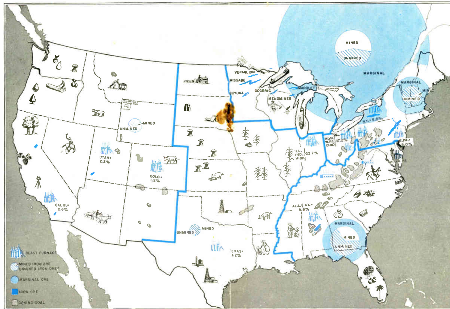
This map gives an idea of the principal areas now producing iron ore, the coking-coal regions, and the concentrations of blast-furnace capacity as percentages of the U. S. total. Circles indicate quantities by regions of mined and unmined ore now considered commercial and rough estimates of marginal ore (data by E. W. Pehrson, U. S. Bureau of Mines). The amount of marginal ore in the Central and Western regions is thought to be small.
