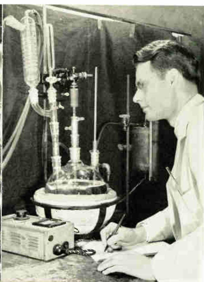
Starting with a water-thin, amber-colored liquid such as is being "brewed" by Mr. Foster, upon polymerization Fosterite becomes a nonporous solid impervious to moisture and resistant to fungus, both vital for tropical insulation.
