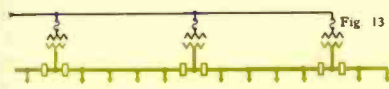
Fig. 13—Protective links on primary side of transformers; internal secondary breakers (two in each transformer tank) for sectionalizing secondaries; no breaker or fuse in secondary leads of transformers. One sectionalizing breaker in
