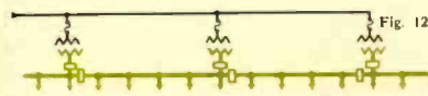
Fig. 12—Protective links on primary side of transformers; internal secondary breakers for sectionalizing secondaries, tripped by current in the low-voltage leads of their associated transformers. Each sectionalizing breaker and its
