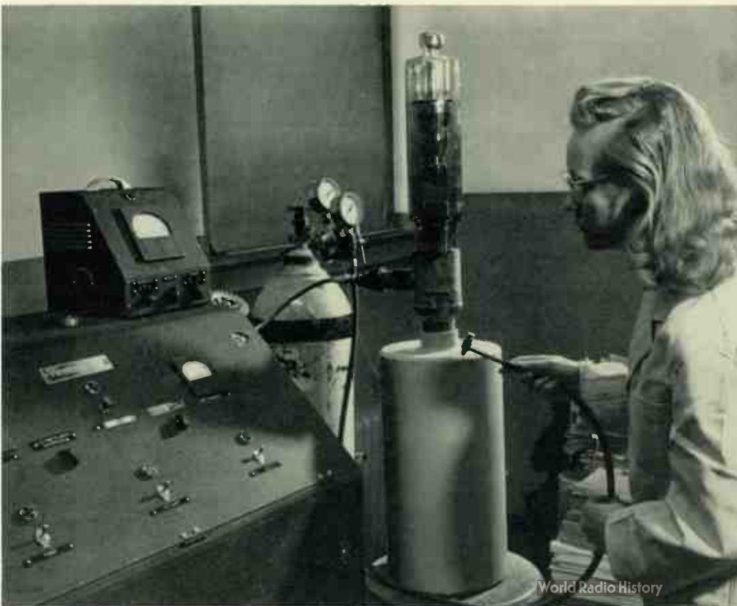
Fig. 1—An operator plays a tiny stream of helium over the evacuated chamber. Small samples of the gas in the vacuum system are drawn off into the mass-spectrometer tube of the leak detector. The tube is set to be sensitive to helium atoms and quickly registers their presence in the system on the recording instrument.
