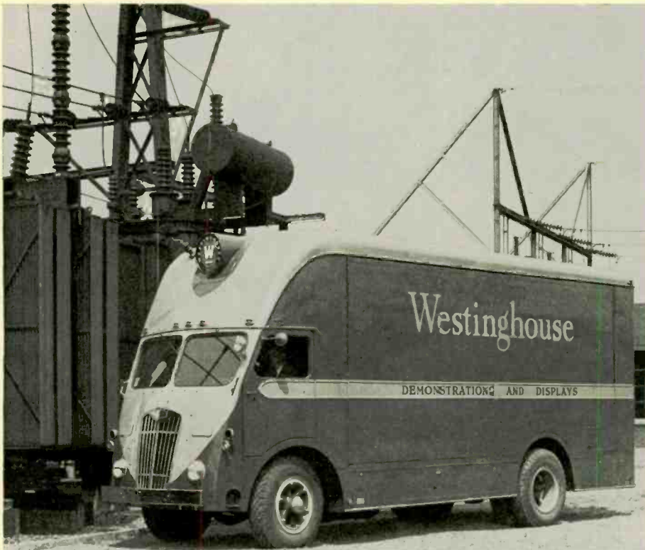
The principles and basic equipments of electric-power distribution and its protection are visibly displayed by a distribution system on wheels. A surge generator makes possible the demonstration of each type of protective apparatus.
