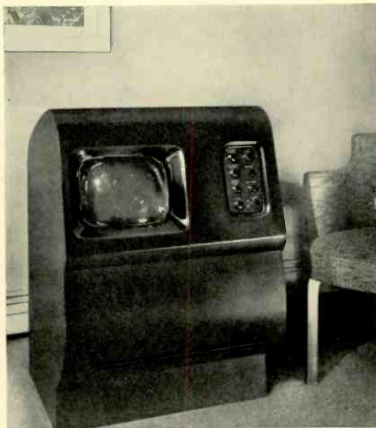
A direct-viewing color television receiver as used in demonstrations by the Columbia Broadcasting System of N. Y.
