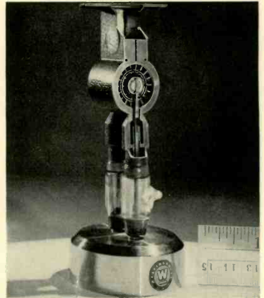
A 3-cm magnetron cutaway to show internal arrangement. The terminals running up from below are for the cathode heater. Power from the wedge-shaped cavities feeds through the vertical slit into the waveguide at the top. A glass window in the flange forms the vacuum seal. To obtain the desired mode of oscillation, alternate cavities are connected by pairs of circular rings.
