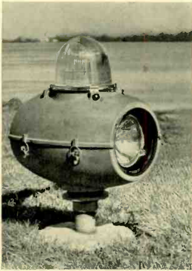
The runway is unmistakably outlined by rows of units of this type. It consists of two powerful incandescent, sealed-beam lamps, for use when visibility is poor, and, on top, one incandescent lamp employed when low-intensity only is required.
