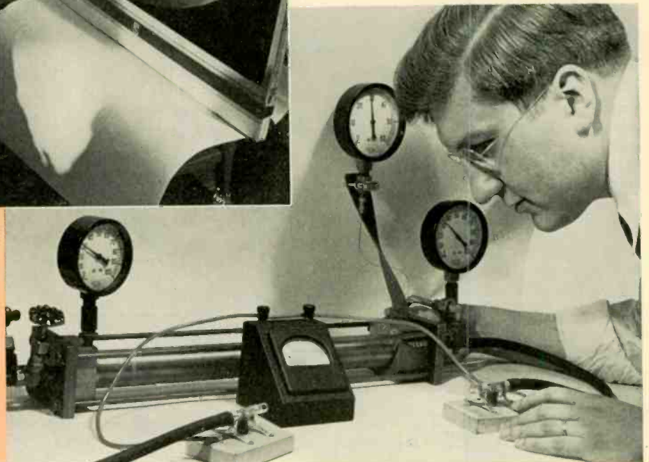
Dr. W. C. Johnston of the Westinghouse Research Laboratories uses this equipment to study flame velocities and combustion rates of jet engines.
