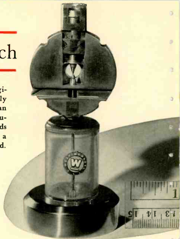
A TR switch (type 1B24) for use at about 10 000 megacycles. The adjustable gap is visible within the coupling windows.
