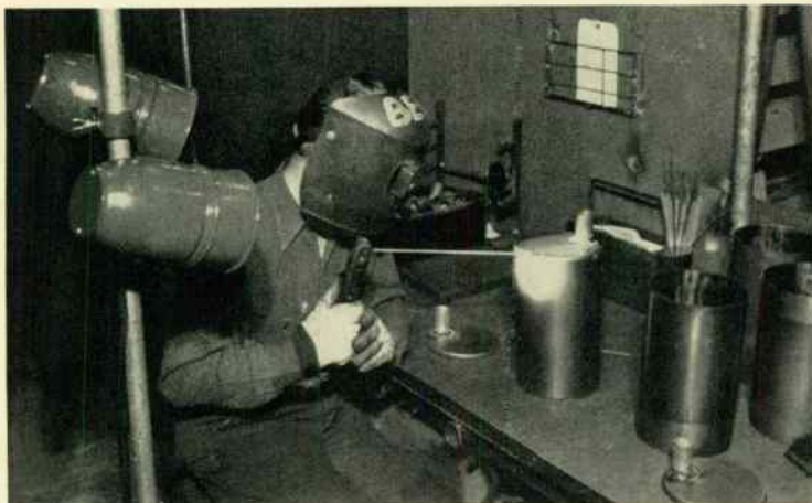
At a three-foot distance the new welding spotlight has a beam five inches in diameter, sufficient for most welding, cutting, or brazing work.
