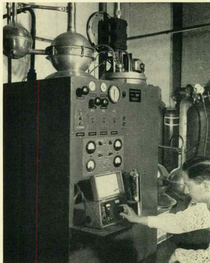
Dr. Aaron Wexler makes a thermocouple measurement on the Collins helium liquefier. He heads up a fundamental research program to explain behavior of electrical and magnetic phenomena at temperatures near absolute zero.
