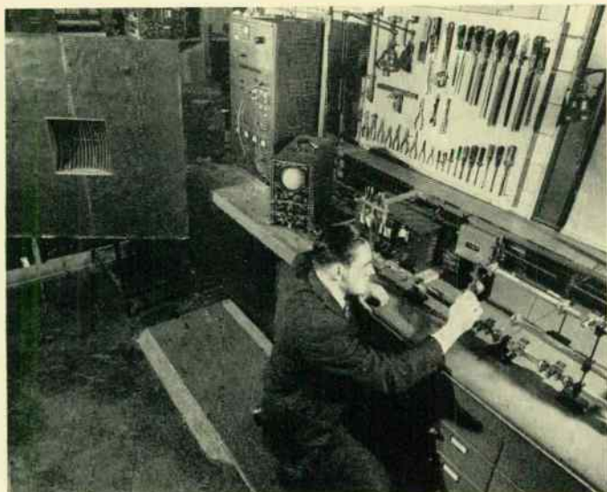
Mr. Duckett adjusts the attenuator of the waveguide system used in the measurement of microwave scattering caused by raindrops. The radar transmitter is to his left. The simulated raindrop is placed on a special screen (lower left) that absorbs radar waves. Waves reflected by the raindrop are picked up by the receiver.
