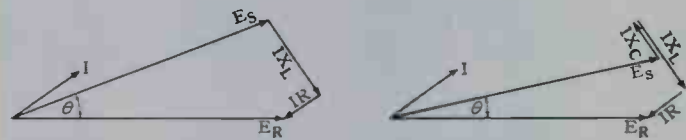
Fig. 3—When the load power factor is leading, a series capacitor is undesirable because it decreases the receiving-end voltage.
