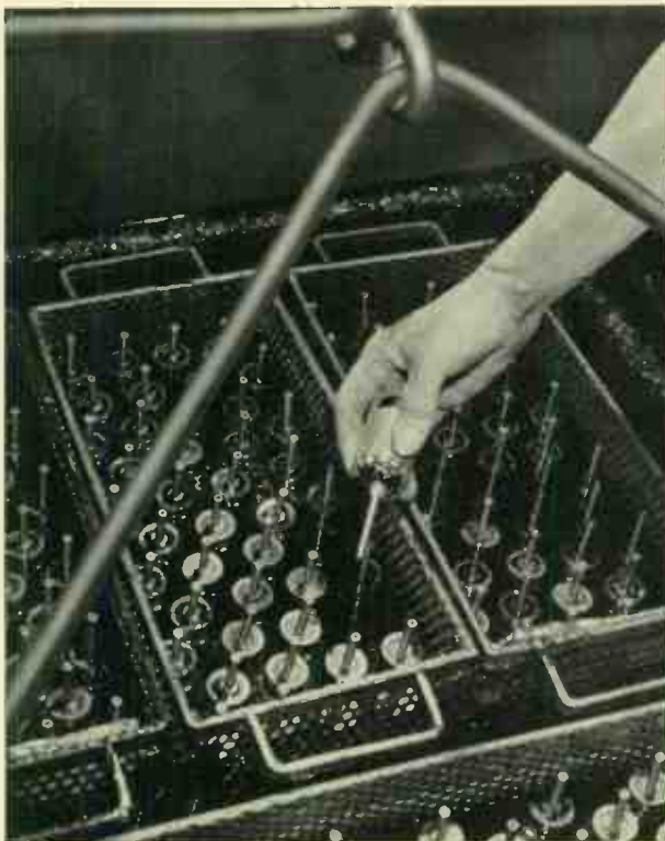
(Left) Armatures for small universal motors, such as used on adding machines, are treated with Thermostat. (Right) A high-voltage coil of a transformer immediately after dipping
