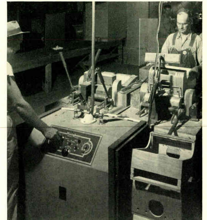
Radio cabinets are glued with the aid of this r-f generator and a special jig.
