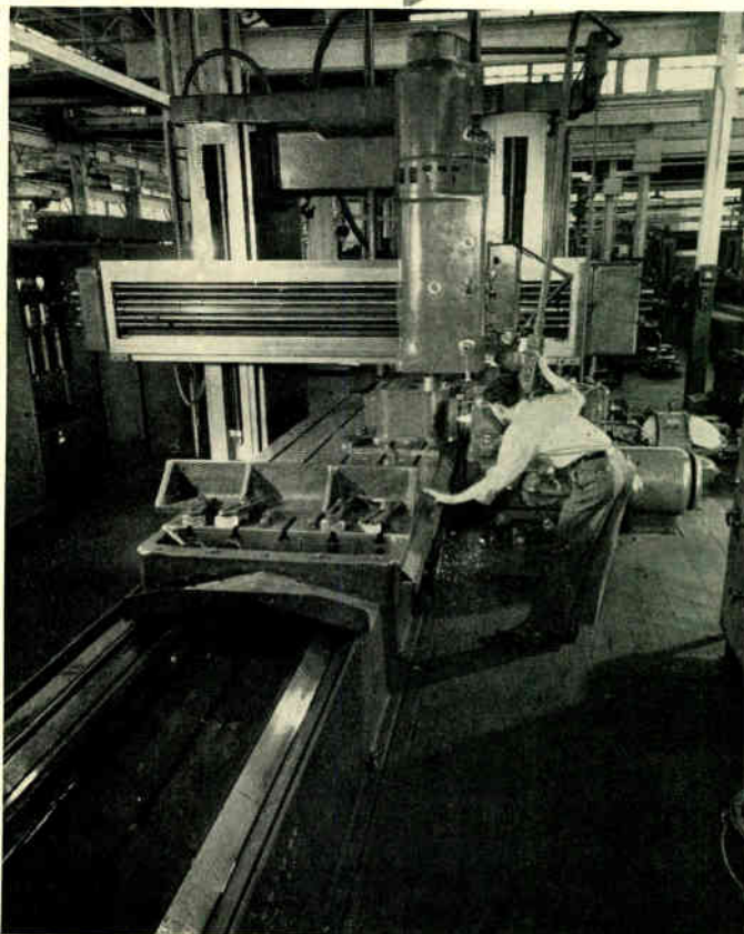
The drive for the table feed of this planer-type milling machine is a 5-hp Mototrol drive. The control cabinet can be seen to the left of the rail; the motor is on the floor to the right of rail (rear motor).
