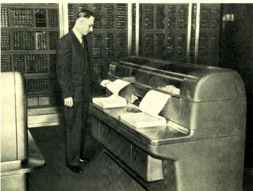
Fig. 4—Printers give a running account of results produced by the IBM calculator.
