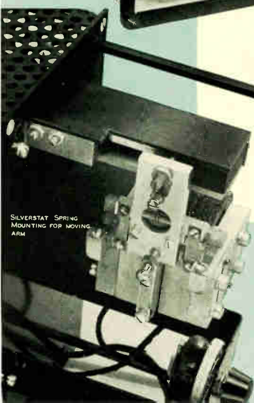
Fig. 4—The spring-mounted moving arm is the main moving element of the Silverstat regulator. This type of mounting entails no wear.
