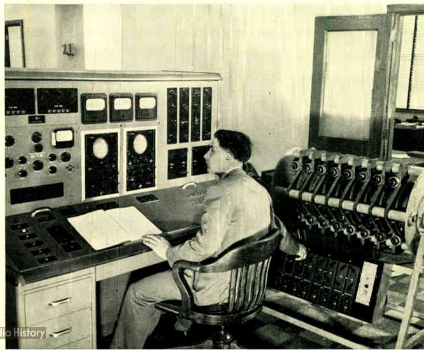
Fig. 9—This rotating synchronous switch is used on the Anacom to repeat transients, to build special forcing functions, and for other analytic purposes.
