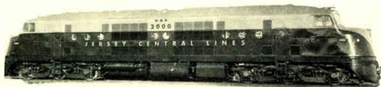
A 2000-hp double-end Baldwin-Westinghouse diesel-electric locomotive for suburban service.
