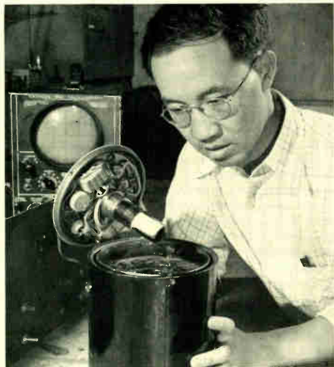
Dr. Kuan-Han Sun inspects the neutron detector. The white coating on the phototube is the uranium phosphor.
