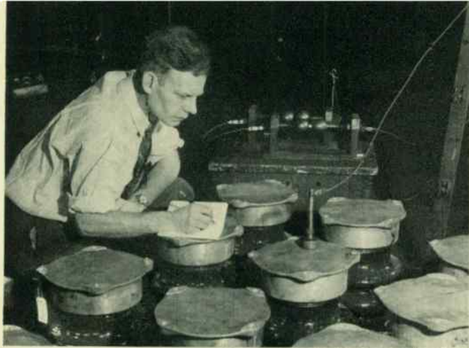
Testing SV lightning arresters for rotating machines.
