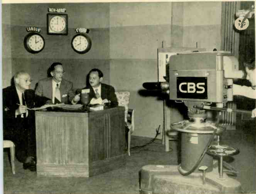
A CBS television camera shows newscasters in action. The camera, with lenses, camera tube, and amplifiers, is mounted on wheels.
