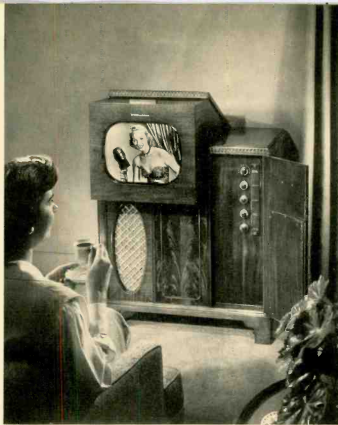
A Westinghouse console-model television receiver. The 12-inch viewing kinescope is lowered out of sight when it is not in use.
