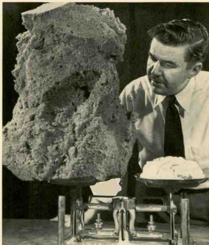
Even fluffy meringue is far heavier than the new foamed resin.
