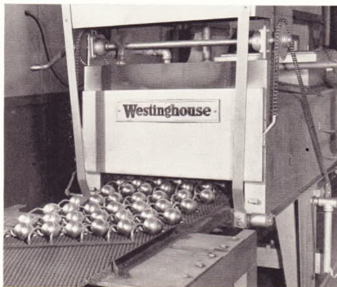
Fig. 5—A channel to support the tube ends positions the assemblies on the woven belt without elaborate supports.
