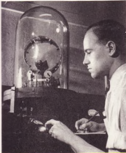
Thin films are deposited on surfaces suspended inside the rotating ring shown in the evacuated glass bell. Mr. T. E. Ebert controls film thickness by timing the deposition.
