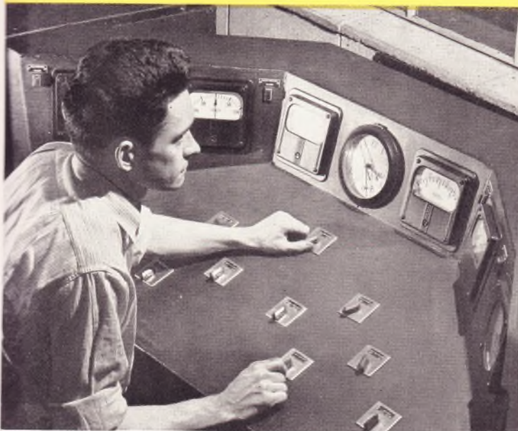
Fig. 5—All controls, indicating instruments, and recording devices are in a centralized room conveniently located to give the operators a full view of the testing area and of the impulse generator. Looking through the window from the test floor (right) one sees the operator at the control desk and behind him is the electronic oscillograph and its operator. The view below is taken looking over the right shoulder of the control-desk operator.
