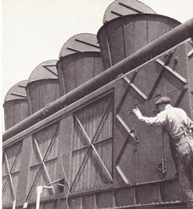
Fig. 4—A view of a condenser car with the tubes exposed.
