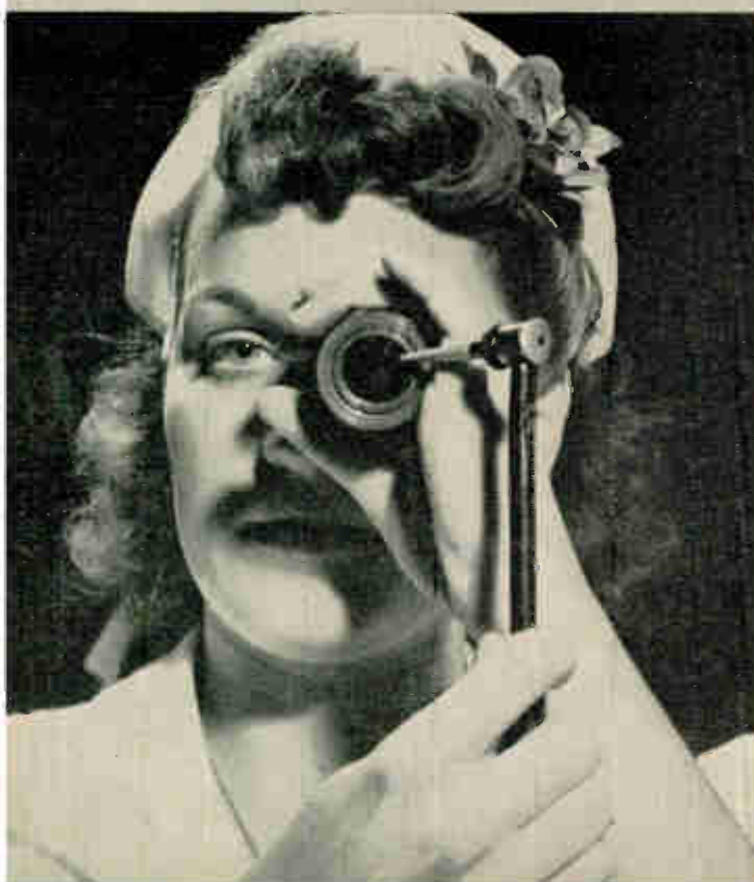
To protect the eyes of gunners who peer through telescopes in tanks jerking over rough ground, Kathryn Gross attaches a rubber-covered shield to the three-power telescopes made at Mansfield. Below: Eileen Swank shows how midget vacuum cleaners with soft paper tips pick all dust specks from the glass discs on which the telescope aiming scales are marked.
