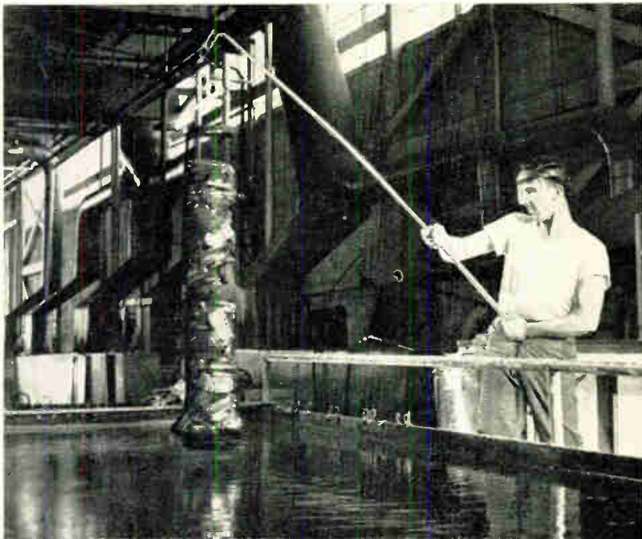
⚡ To help toughen their aluminum surface, warplane nose ribs get a bath in water at a 50-degree temperature. Gordon McElroy is shown fishing up a basket of the ribs, which will go into elevators for a Thunderbolt.
