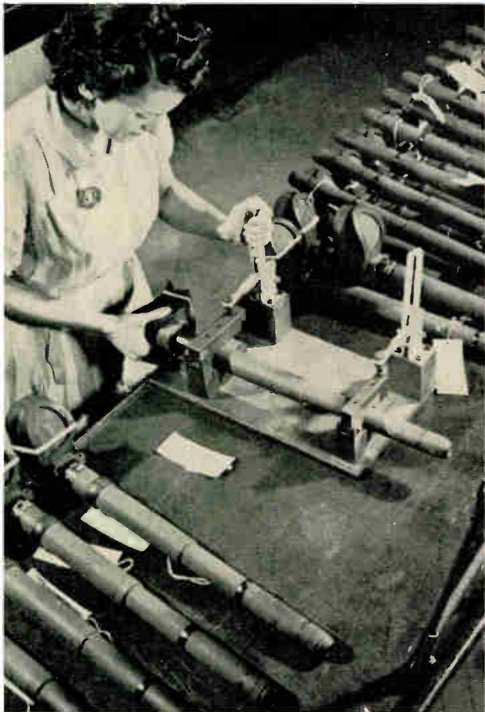
To protect the eyes of gunners who peer through telescopes in tanks jerking over rough ground, Kathryn Gross attaches a rubber-covered shield to the three-power telescopes made at Mansfield. Below: Eileen Swank shows how midget vacuum cleaners with soft paper tips pick all dust specks from the glass discs on which the telescope aiming scales are marked.
