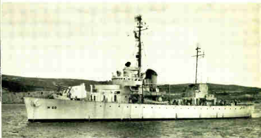
Above is the Coast Guard cutter Campbell . It is the largest of cutters, and, powered with 6200-shp geared turbines, has a range of 8000 miles. At right is the Androscoogin , a turbine-electric ship used in North Atlantic weather patrol.
