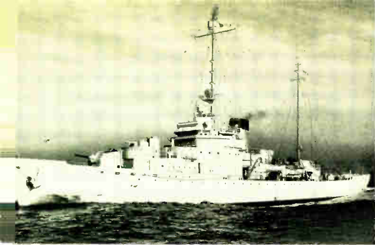
Above is the Coast Guard cutter Campbell . It is the largest of cutters, and, powered with 6200-shp geared turbines, has a range of 8000 miles. At right is the Androscoogin , a turbine-electric ship used in North Atlantic weather patrol.
