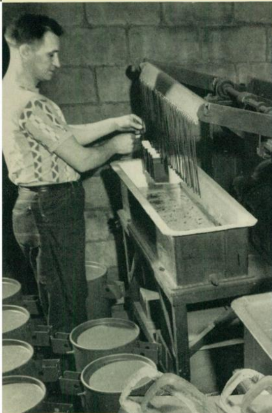
← Fig. 8—This equipment dips test panels into a bath of either acid or alkali and then lifts them out of the solution to dry in air on a four-hour cycle—two in the solution followed by two in the air.
