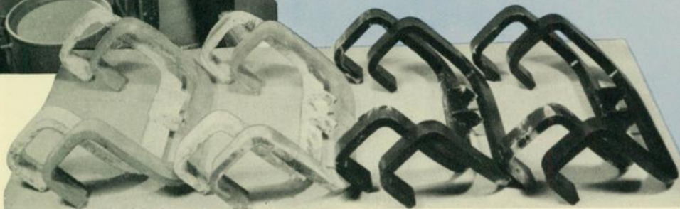
← Fig. 10—Various finishes on hanger irons were exposed to 2000 hours of salt spray. From left to right the finishes are: galvanized; cadmium plated; galvanized and bonderized; cadmium plated and bonderized; galvanized plus mica-base finish; cadmium plated plus mica-base finish; galvanized and bonderized plus mica-base finish; and cadmium plated and bonderized plus mica-base finish. Only the cadmium-plated and bonderized plus mica-base finish hangers (at extreme right) showed no signs of attack.
