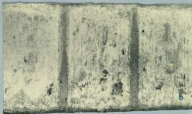
Fig. 5—(a) Burning of filler pieces and (b) surface deterioration of waterwheel-generator insulation.
