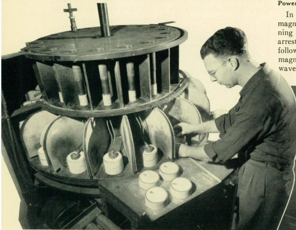
Fig. 1—This revolving surge-testing table is being loaded with station-type lightning-arrester blocks. The surges are introduced to the specimen blocks at the back of the machine through the contacts that can be seen on top, above each cubicle. The series gaps are inside the white rings seen above each test cubicle.
