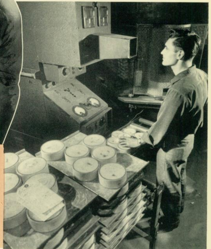
Fig. 1—This revolving surge-testing table is being loaded with station-type lightning-arrester blocks. The surges are introduced to the specimen blocks at the back of the machine through the contacts that can be seen on top, above each cubicle. The series gaps are inside the white rings seen above each test cubicle.
