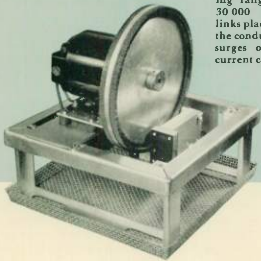
Fig. 6(a)—The fulchronograph uses magnetic links to measure current. The rotating wheel adds time to the record so that wave shape and duration of the surge can be determined.
