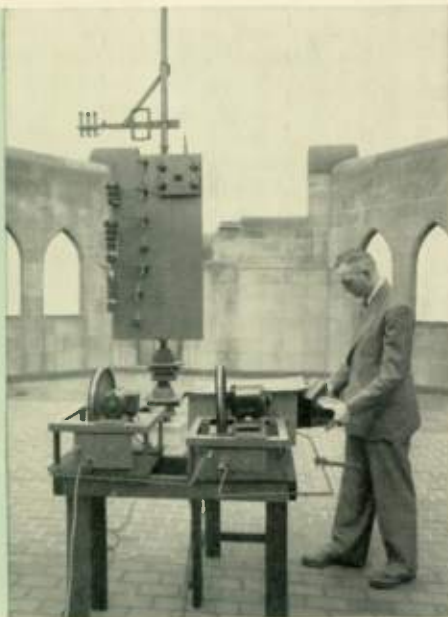
Fig. 9 — This is the direct-stroke lightning station on the roof of the Cathedral of Learning. Dr. E. L. Harder is placing the photographic recorder in its protective house. A high-speed and a slow-speed ful-chronograph are evident on the table in the foreground. Surge-crest ammeters, a surge-front recorder and an automatic cathode-ray oscillograph (not shown in the picture) are also used at this station.
