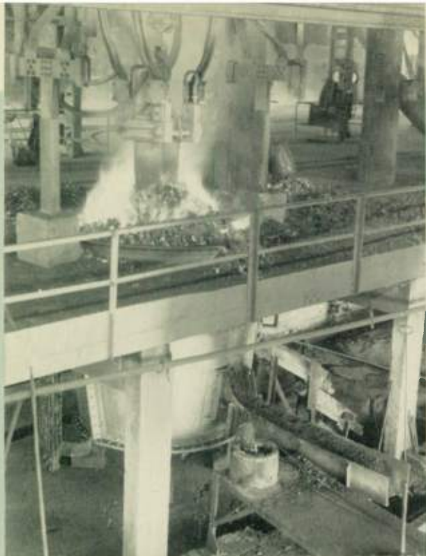
Cobalt-copper concentrate is reduced to liquid metals in electric furnaces like this in Africa. Photos courtesy Union Minière du Haut-Katanga.
