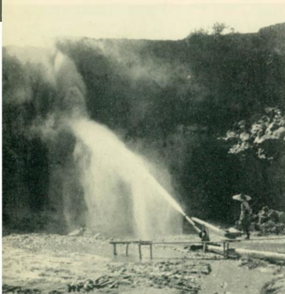
← In the Far East powerful jets of water wash down banks of gravel containing tin-bearing particles.
