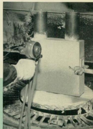
Zinc, vaporized by heat, is sprayed onto a capacitor case, giving good weather resistance.
