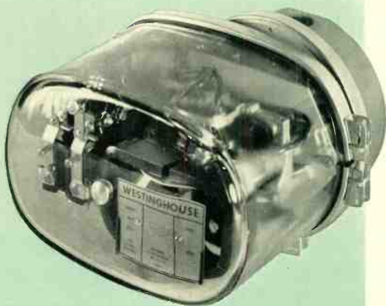
Fig. 7 — The type CJ-2 socket-mounted, induction-disk type voltage control. No additional devices are needed when this relay is used with an oil contactor or a CSO-1 switch.
