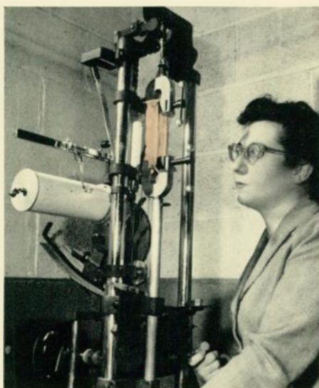
This apparatus is used to detect any change in the tensile strength of the cloth during washing. Cloth is placed between clamps so that the upper and lower jaws pull on the same vertical threads. The cylindrical graph records tensile strength.
