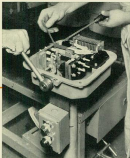
Fig. 3—The master switch used on the log-carriage drive.
