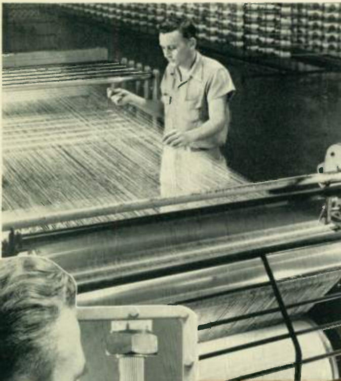
Filaments of acetate are born at the left, where the operator watches them emerge from the spinneret into an updraft of warm air that evaporates the acetone. In the view above hundreds of acetate yarns are wound onto a beam. At right are containers of purified wood pulp or cotton linters awaiting manufacture into acetate. Photos by Tennessee Eastman.
