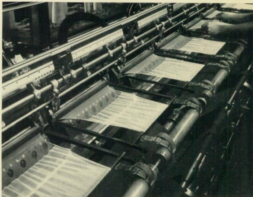
One of the most complex precision-manufacturing devices in all industry is the full-fashioned hosiery knitting machine. Here are 32 "Cameo" brand stockings, in the early stages, being knit simultaneously and automatically in a Burlington Mills factory.
