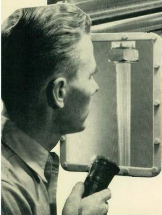
Filaments of acetate are born at the left, where the operator watches them emerge from the spinneret into an updraft of warm air that evaporates the acetone. In the view above hundreds of acetate yarns are wound onto a beam. At right are containers of purified wood pulp or cotton linters awaiting manufacture into acetate. Photos by Tennessee Eastman.
