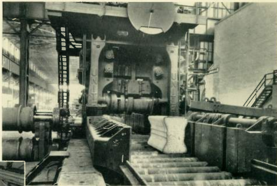
Fig. 8—A 7000-hp reversing mill twin drive with 3500-hp, 35/80-rpm main-drive motors (background), and a flywheel m-g set and liquid slip regulator.
