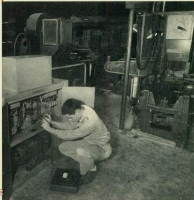
Fig. 17—Electronic edge-position regulator for a side-trimming line. This is typical of recent electronic regulators.
