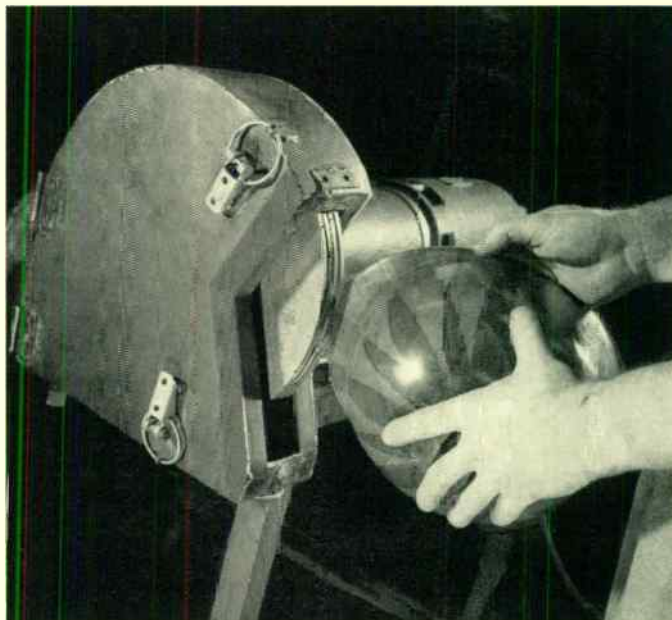
The new laminated burnishing wheel being used to finish the edges of a helmet liner. Grinding is done in the grooves of the wheel.
