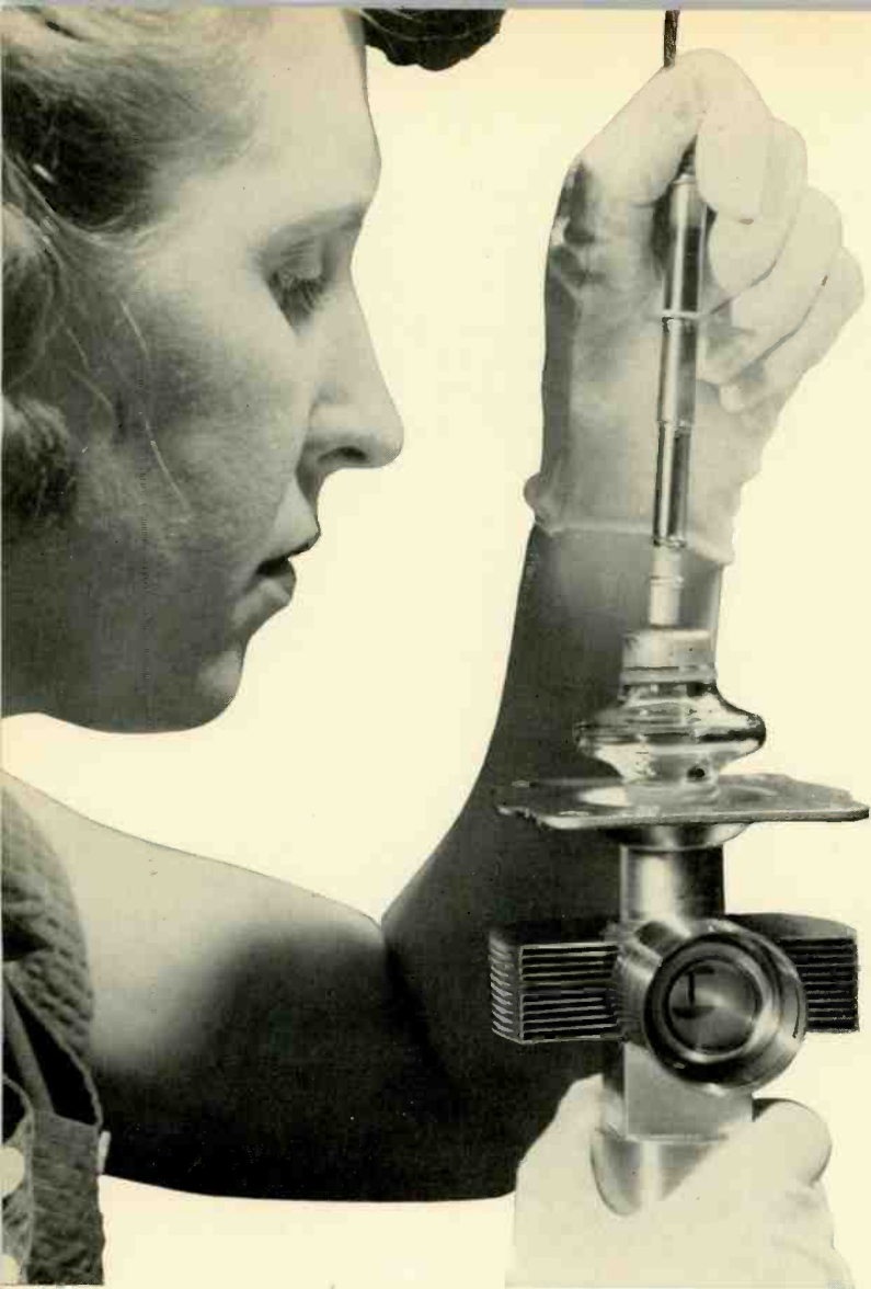
Cermet Cathode —An indirectly-heated cermet cathode being installed in a magnetron (WL-6249). The cathode proper is the smaller cylindrical section about \frac{3}{8} inch long, which is located about \frac{1}{2} inch from the free end of the cathode-mount assembly.
