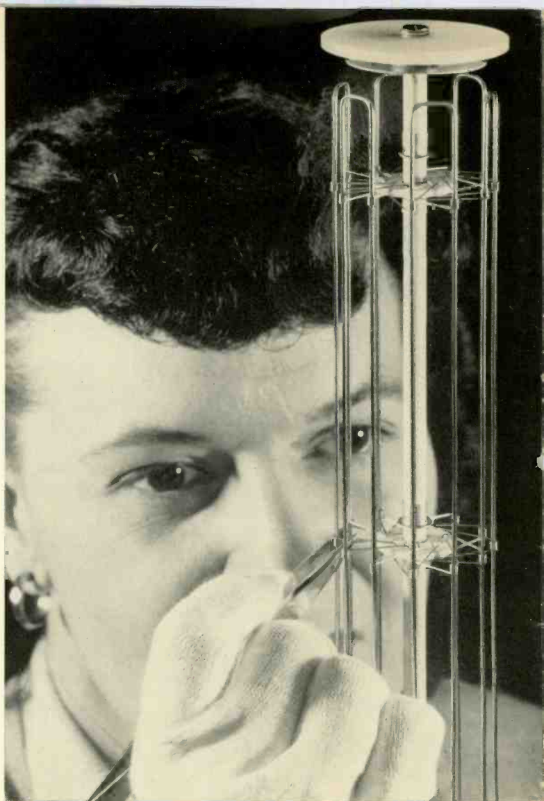
Spider Insulator —This newly-designed spider insulator holds filament strands from moving radially in the WL-5936 triode.
