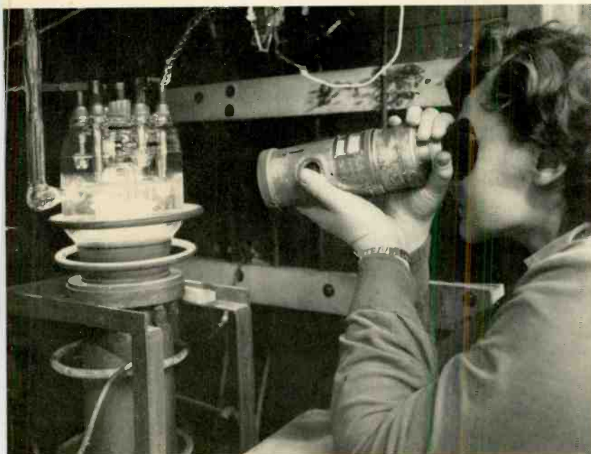
Flying Leads on this tube (WL-6623 on the left) provide for electrical circuit connections with a minimum of resistance losses.
