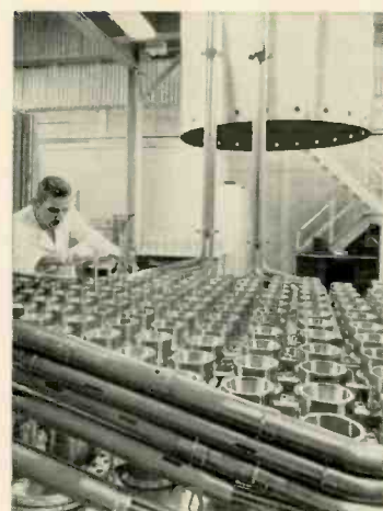
Stainless steel is much in evidence in the PWR plant, as witness these parts of the nuclear reactor core.
