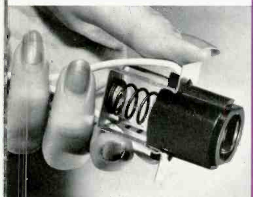
Above —This new fluorescent lamp-holder can provide for three different lamp types—bi-pin, slimline, or recessed contact types. Three different plungers, with identical external configurations and mounting dimensions, fit interchangeably into one basic bracket.
