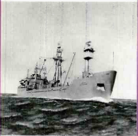
The USNS Eltanin , a cross between a cargo ship and ice breaker, has already proven herself in Arctic maneuvers. Built by Avondale Marine Ways, Inc., at New Orleans, the ship is propelled by a diesel-electric variable-voltage system. Each of the two 1350-shp. double armature d-c propulsion motors is directly connected to one of the twin propellers.
