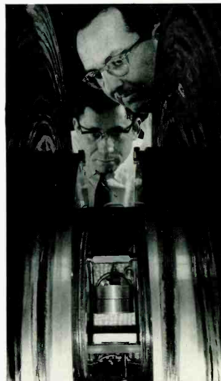
NMRAA —In the small metal box between the poles of this large electromagnet, scientists vibrate the atoms of a crystal up to 20 million times per second to study the structure of crystal matter (story at left).
