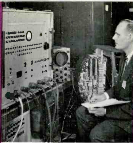
Engineer takes test data from an automatic Computer Test Set.
