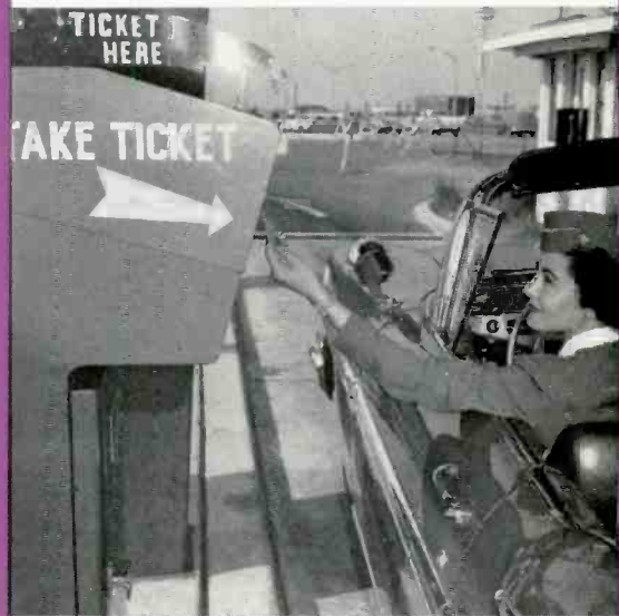
Above—An offbeat but appropriate Cypak control application this year is at New York International Airport's parking lot. As a driver approaches the lot, a magnetic coil beneath the road causes the ticket dispenser to stamp the date and time on a ticket. As the driver takes the ticket from the machine, the parking lot gate raises. The gate closes as the car passes over a second coil.
