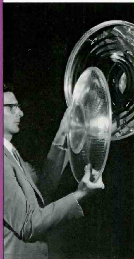
This new experimental luminaire is designed for lighting superhighways, with the light beam thrown along the road in the direction of traffic flow. Interior louvers plus lens are designed to provide sharp cutoff of light in other directions.
