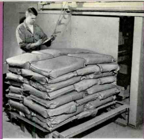
Though bags make a handy container, the full bags are difficult to handle. But this Cypak controlled Miller bag palletizer automatically stacks interlocking layers of bags into a neat easily handled pile. The Miller Engineering Corporation is located in Louisville, Kentucky.
