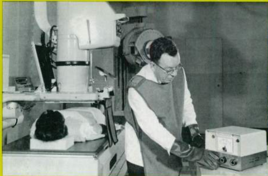
The Radometer, a new device for measuring x-ray dosage to a patient during fluoroscopy, spot-film radiography, or cineradiography.
