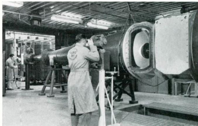
Runs exceeding escape velocity last but one-tenth of a second in Tunnel Hotshot II, which is part of the Gas Dynamics Facility at the Arnold Engineering Development Center. Longer runs would damage or destroy components or the tunnel.
