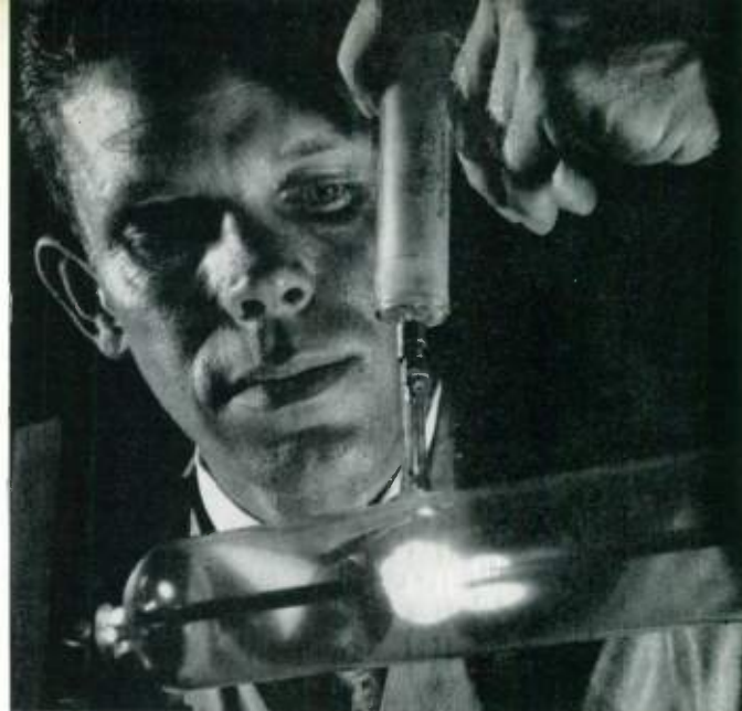
The effectiveness of SF_6 as an arc-quenching medium is demonstrated by this simple laboratory experiment. A high-voltage arc is readily drawn when the tube is filled with air, but is extinguished when a small amount of SF_6 is injected into the tube.
