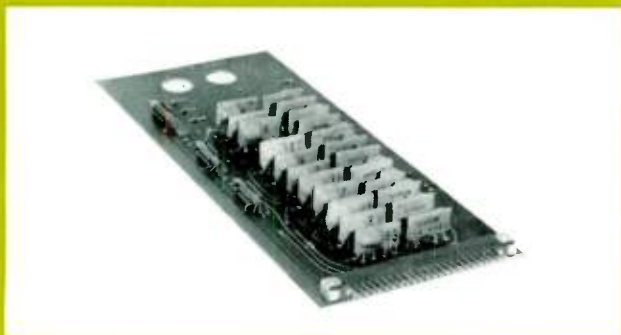
Fig. 8—Printed circuit boards on which NOR units are assembled.
