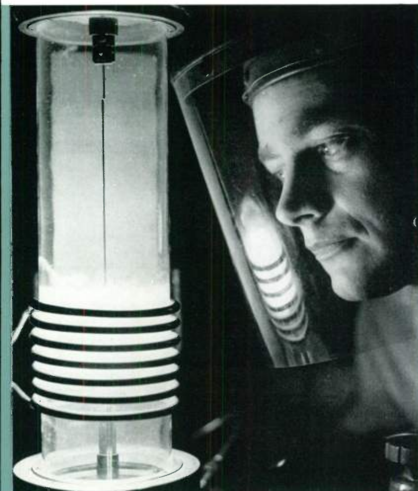
A ribbon-like crystal of germanium rises out of a molten pool in this crystal-growing furnace at the Westinghouse research laboratories. Such thin, flat strips are the exact form in which germanium is used in making transistors and other semiconductor devices. Therefore, they require none of the costly, time-consuming cutting and grinding that wastes up to 80 percent of conventional ingots of germanium.
