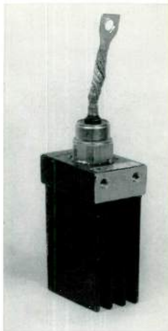
Fig. 6 (left)—Typical silicon cell for voltage ratings up to 500 peak inverse volts. (Right)—Cross sectional view of silicon rectifier assembly.
