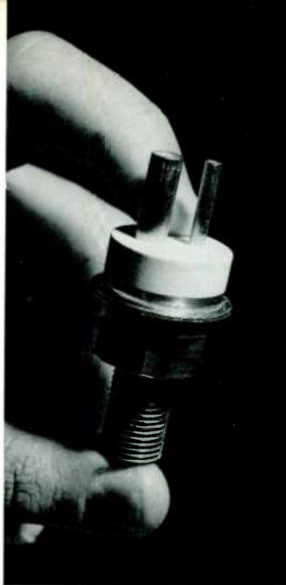
Up to 5 kw of power can be controlled when this silicon transistor is operated as a switch.
