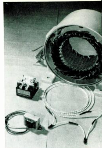
Fig. 7 (right) —A typical PTC thermistor harness assembly for a three-phase winding.
