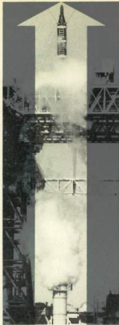
At top of its trajectory, missile is snubbed by modified carrier arresting gear.
