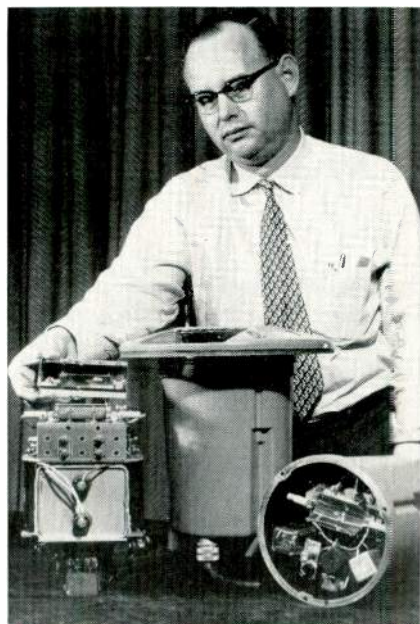
This flush-mounted flashing light has power supply and lamp assembly in one compact unit.
