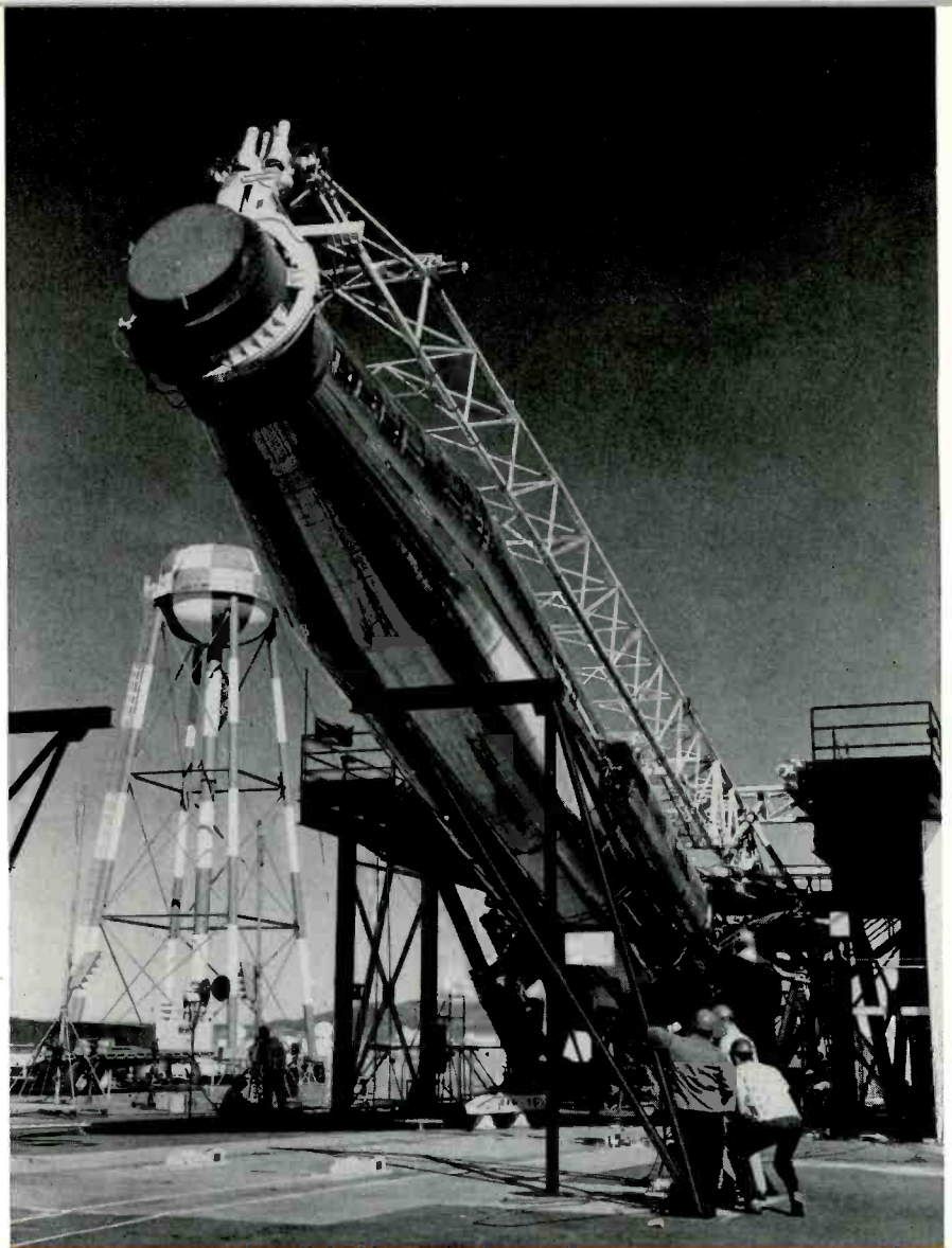
Shown in operation is the Atlas missile erector, which can raise a missile from a horizontal to a vertical firing position in a matter of minutes.
