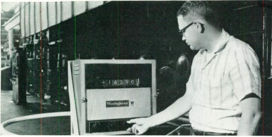
Control unit of the digital draw and speed indicator at the Pensacola Mill of the St. Regis Paper Company.
