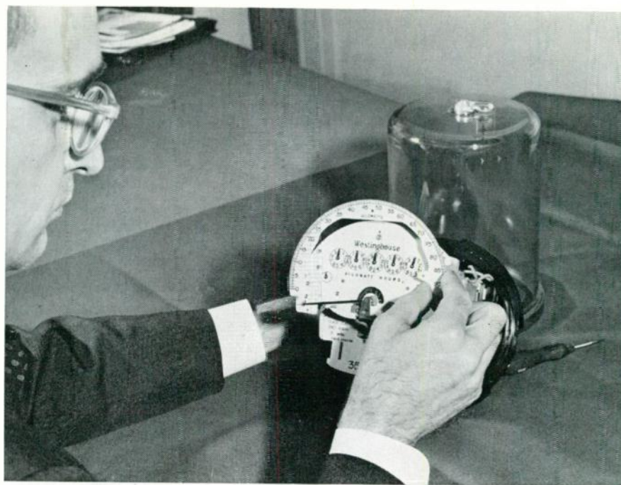
One side of this Mark I demand register scale reads 0 to 96 kilowatts; the other side reads 0 to 48 kilowatts. The tab at the right depresses a pin that shifts the register's gears to the high range when the scale is installed in this position.
