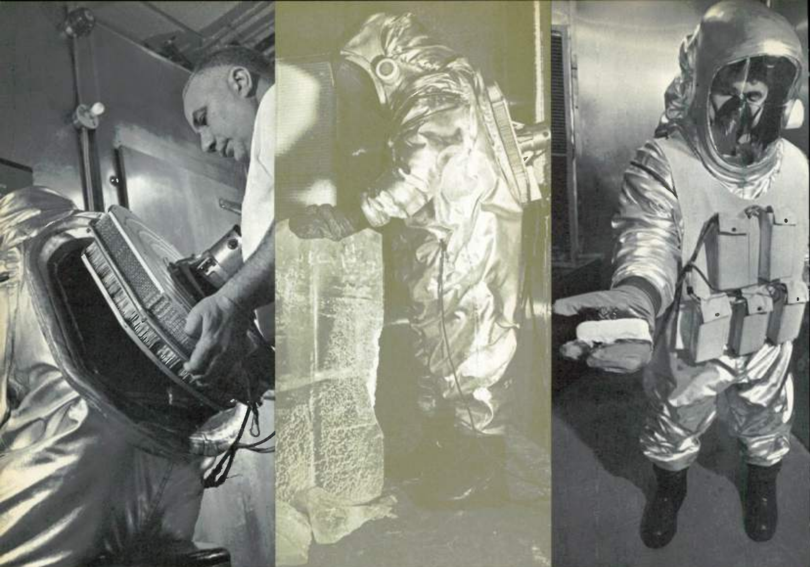
This new experimental Navy climatic suit is heated or cooled with a thermoelectric air-conditioning unit (Left). A temperature of about 80 degrees F is maintained inside the suit when outside temperatures are 40 degrees below zero (Center) or 135 degrees above (Right).
