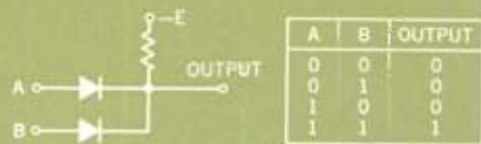
Fig. 7 (a) Diode circuit for producing negative logic AND. Both inputs A and B must be present to produce output, as shown in the table. (b) The diode matrix is one form of decoding matrix. As shown in the accompanying table, an x-output wire can be energized by providing an AB input word. (c) This functional diagram illustrates the method of selecting words from memory. The memory address word is placed in a memory address register (some form of flip-flop register); this register energizes the x- and y-selection matrices, which cause the word to be selected from memory and placed in a memory output register.
