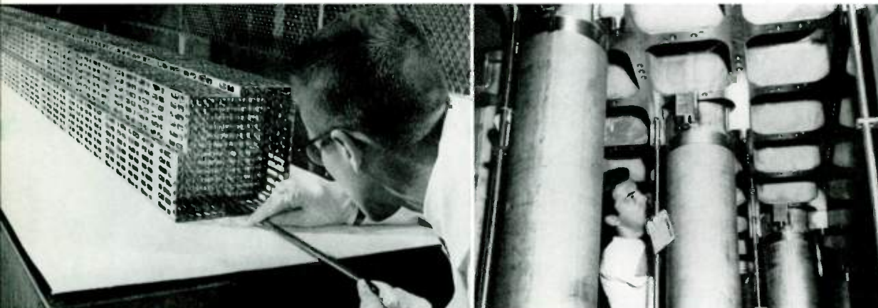
Fig. 6 (Far left) A spring-clip fuel assembly. The grids have spring fingers, which grip the fuel rods.
