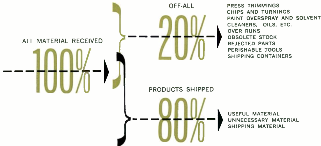
Fig. 2 A typical breakdown of raw material distribution. Note that some unnecessary material is found in the product itself, as well as in the discarded material. The term "off-all" refers to that part of the material received in a plant that is either taken off or not used as a part of the product shipped.
