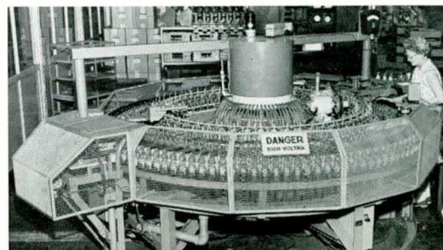
Fig. 7 (Below) This machine calibrates, tests, and classifies small circuit breakers automatically at a rate of 400 per hour.
