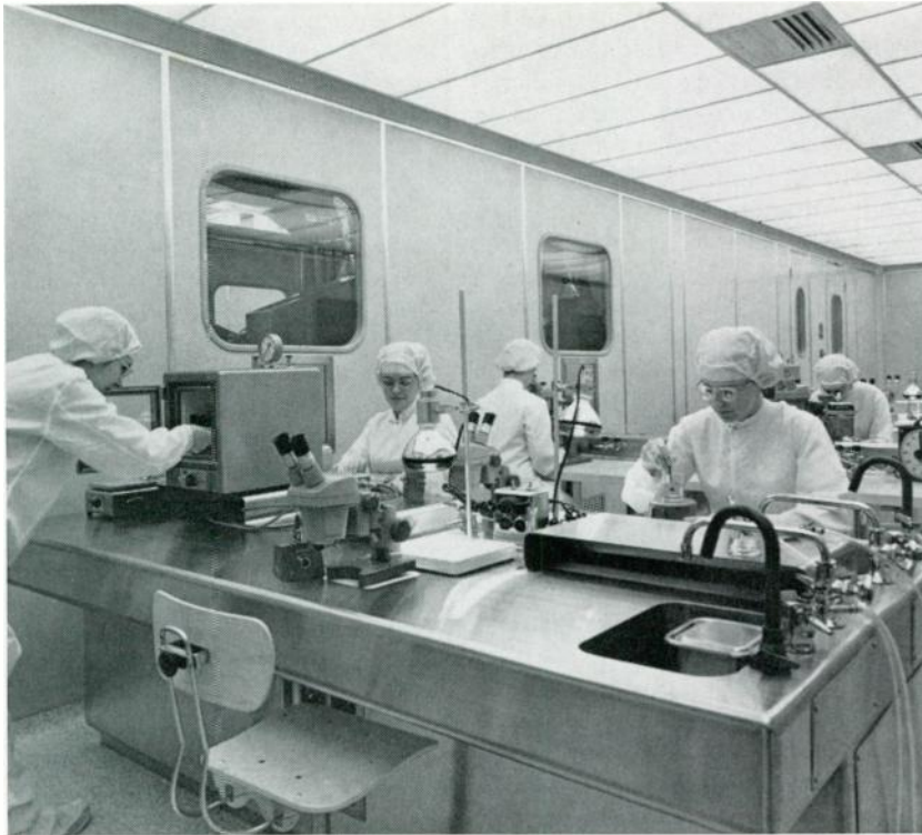
Interior view of typical clean room, used in making molecular electronics devices.
