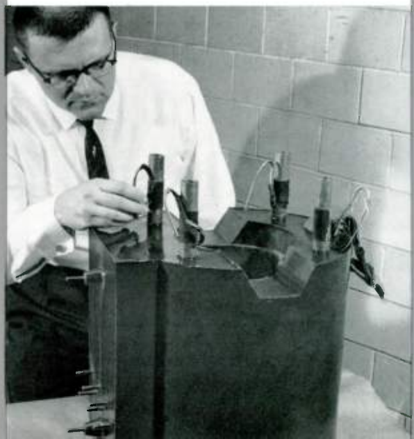
Fig. 2 (Above) At left is a model coil, and at right a prototype coil for a 500-kva 15-kv transformer. (Below) Another view of the prototype coil.
