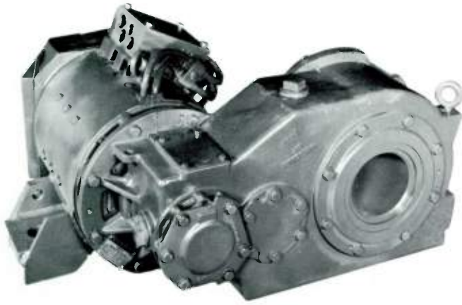
This motor and gear unit accelerates and brakes rapid-transit cars, yet is small enough to be mounted on a car truck.
