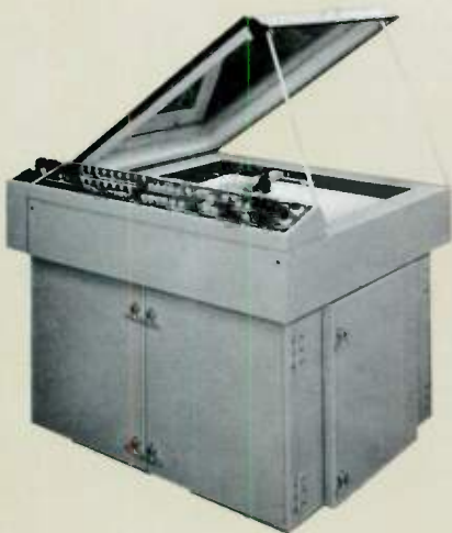
Fig. 1—The Autoplot console consists of a digital computer in the base, and a plotter on top. The master control panel governs operational mode selection, and the insertion of operational constants, such as the geographical coordinates of the navigational reference stations and chart scale factor.
