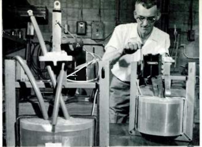
The complete core-and-coil assembly for the Capaciformer. The core is a conventional Wescor design.
