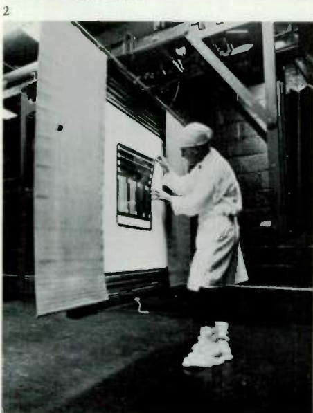
(1) An optical pyrometer is used to take a temperature profile during an epitaxial growth operation. (2) Masking slides are produced with a tolerance equal to only a fraction of the width of a hair. The operator is mounting a pattern that will be photographed and reduced from several square feet to about the size of a pinhead. As many as 150 copies of this reduced pattern are reproduced on a single plate about the size of a quarter. (3) A silicon wafer, which has been coated with a photosensitive material, is exposed to light causing portions of the photosensitive material to harden, and leaving the shaded portions in a condition for further processing. (4) Silicon dice, or chips, as small as 0.05 inch square are mounted into transistor packages. (5) After mounting and prior to encapsulation, integrated circuits are checked for voltage-current characteristics and for proper connections.
